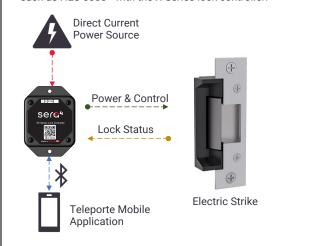
The X-Series controller is powered from a DC source. See Power Requirement section below.
