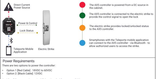
An AC to DC converter is required if there is only AC power available.
